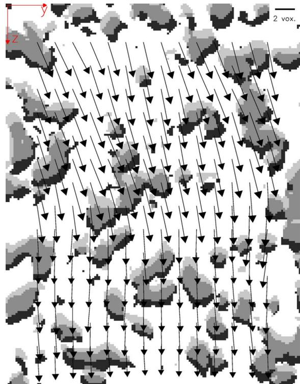
Figure 3: The apparent displacement of the structure during 8 hours, calculated with a 3D algorithm. Light gray areas denote sublimated ice, dark areas signify deposited ice. The size of the slice is  $2.12 \times 2.95 \text{ mm}^2$ .
