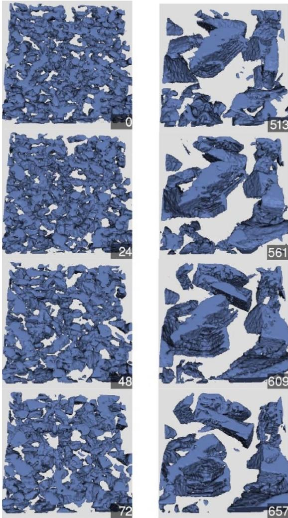
Figure 1. Structural evolution of the sample under a temperature gradient of  $50 \text{ K m}^{-1}$ . The subvolumes have dimensions  $3.6 \times 3.6 \times 0.9 \text{ mm}^3$ , the numbers indicate time in hours.
