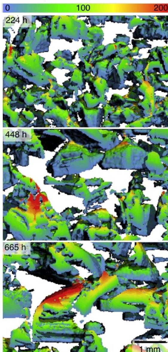
Figure 4. Visualization of the residence time at different stages of metamorphism. The young ice is found on the bottom where the crystals grow, while the “old” ice is found at the top where the crystals sublimate.
