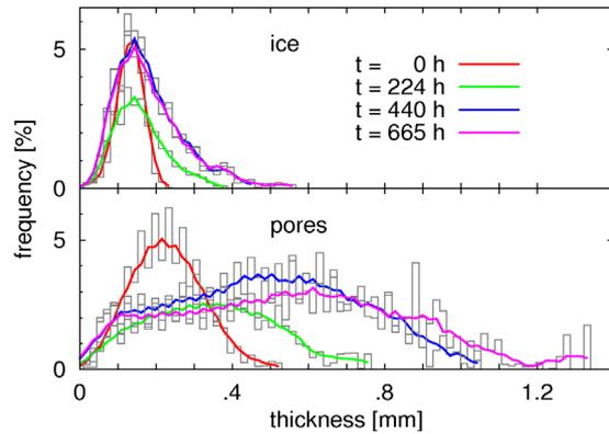
Figure 2. Evolution of ice thickness and pore size of the sample shown in Fig. 1.
