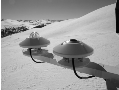
Figure 2 Broadband solar (K&Z CM21) and longwave (K&Z CG4) sensors at alpine tower, Senator Beck basin.
