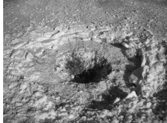
Figure 9. Resulting crater from Shot 2, surface, blasting cap up.
