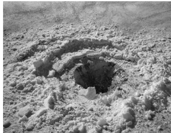
Figure 10. Resulting crater of Shot 3, surface, blasting cap down.
