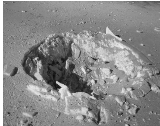
Figure 11. Resulting crater of Shot 4 blasting cap up buried at 0.5 meter below surface.
