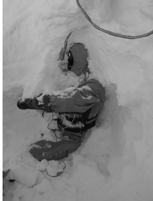
**Figure 4.** Front view of a subject during extrication from burial showing the AvaLung breathing device.
