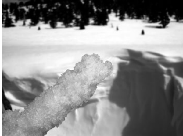
Figure 2. A sample of faceted basal layer grains extracted with a snow corer, March 2006. The core is about 5 cm in diameter. Photograph by Randall Osterhuber.
