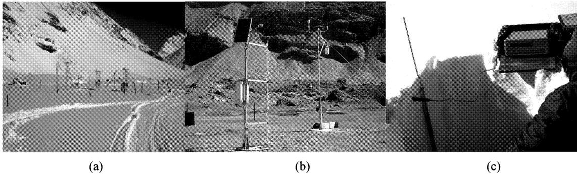
Figure 1. Detail of Patsio site (a) Complete view of Patsio observatory (b) MTX (company name) automatic weather station (c) Thermal conductivity of snow being measured in snow pit
