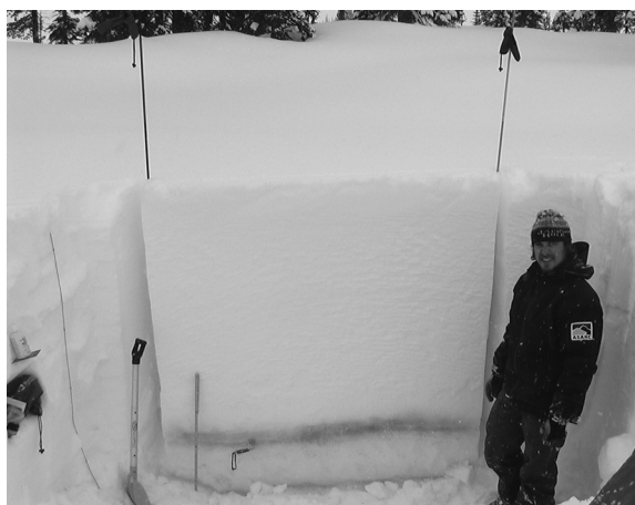
Photo 1. Example of the field test configuration on horizontal terrain. The weak layer is highlighted with contrasting colour. (ASARC Photo)
