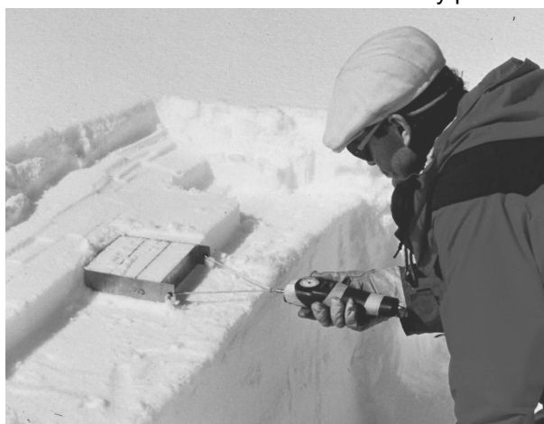
Figure 2. Photograph illustrating a shear frame test being used in a level study plot. A pull gauge, attached to a 250 cm 2 frame, records the maximum force required to produce a fracture in a weak layer when pulled rapidly, parallel to the weak layer.
