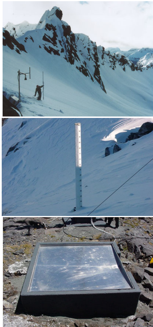
Figure 2: Rover (a) is a mobile station that can be moved to sites of special interest during the season. A down-looking sonic ranger measures changes in snow depth. Snow temperature profiles are measured using thermocouples mounted at 12cm intervals along a pole (b) and multiplexed to a data logger. Rover is anchored to rock, and creep is measured by running a cord around a rotary potentiometer downslope to a glide shoe buried in the near-surface snow. A lysimeter at 1600m (c) measures water outflow from the snowpack. Summer photo shows the 2mx2m catchment tray; typically 3-5m of snow accumulates on top of the tray in winter. A tipping-bucket gauge measures outflow. Antifreeze is pumped into the outflow-orifice to prevent freezing; antifreeze contributes 0.031mm every 3 hours to the outflow.
