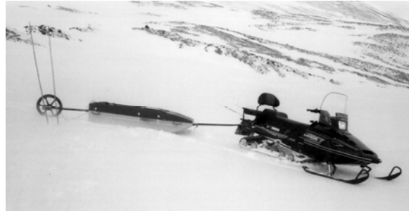
Figure 3: The radar behind a snow mobile during measurements on Spitsbergen spring 2000.
