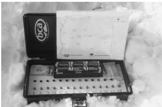
Beacon Basin control panel.
