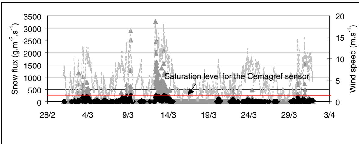
Figure 5 : Comparison of snowdrift direct measurements from two different acoustic sensors during March 2004. Grey triangles stand for data from Flowcapt, whereas dark symbols represent the measurements from the Cemagref sensor.
