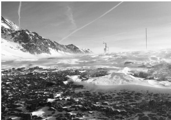
Figure 1 : The “Col du Lac Blanc” altitude station during a snowdrift event. On the left “Grandes Rousses” range rises above the snow-covered pass. The sky line is disturbed by the measurement mast and a graded stick devoted to snowpack thickness measurements. A typical erosion area can be observed in the foreground.
