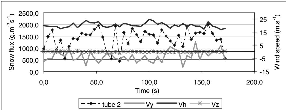
Figure 6 : Fast recording of transport rate and wind speed at “Col du Lac Blanc” station. The line with stars, which stands for the z-component of the wind velocity collapses with the abscissas-axis. The transport rate (dotted line) shows very important fluctuations whereas the horizontal wind speed (dark line) does not vary too much.
