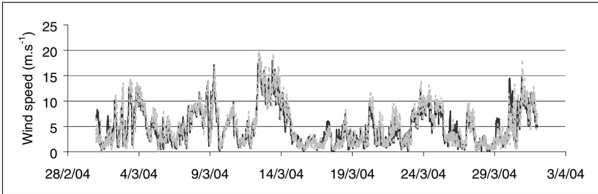
Figure 3 : Comparison of field data from Cemagref (USA1 – grey line) and Météo-France (Young anemometer – black line). The recording consists in 15 minute averaged wind speed during March 2004.
