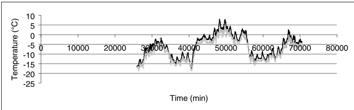
Figure 4 : 15 minute averaged temperature from Usa1 (grey line) and TT100 platinum probe (black line) during March 2004. Time is here given in minutes, 00 minutes corresponding to February 12<sup>th</sup> 14:45.
