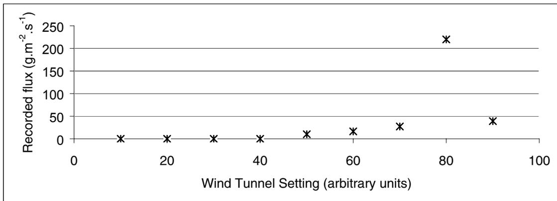
Figure 8 : Maximum recorded flux by Flowcapt during a wind-tunnel experiment without any particles. Samples were taken every five seconds in every tube. Each setting of the wind-tunnel lasted one minute. The maxima plotted here have been selected among all samples and all tubes. Except an isolated point recorded by tube 1 at more than 200 g.m<sup>-2</sup>.s<sup>-1</sup>, no sample overflowed 50 g.m<sup>-2</sup>.s<sup>-1</sup> indicating negligible sensor perturbation.
