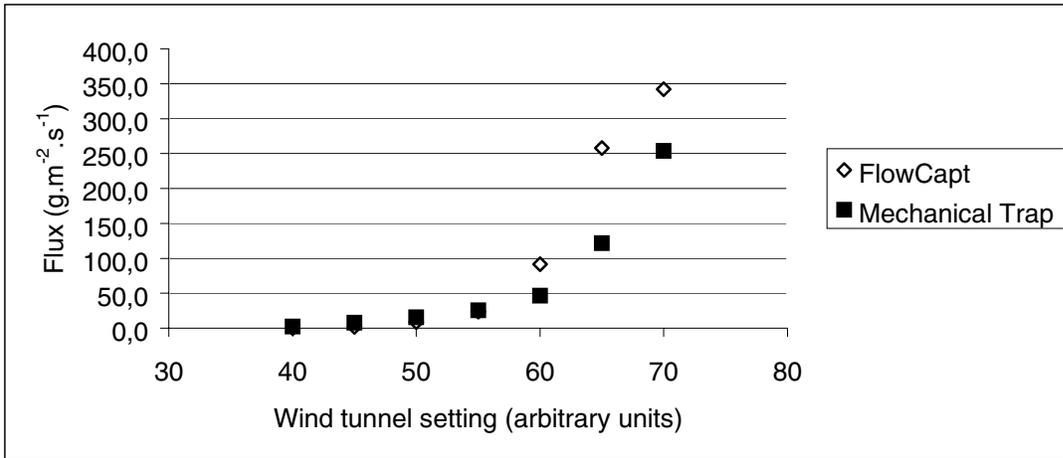
Figure 9 : Comparison of the measurements performed by FlowCapt and a sand trap in a wind-tunnel with sand. A slight overestimation from FlowCapt seems to characterize this graph.
