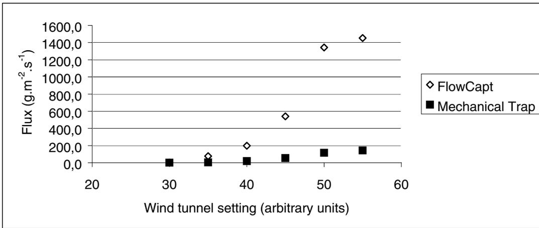
Figure 10 : Comparison of the measurements performed by FlowCapt and a sand trap in a wind-tunnel with corn dust. The overestimation performed by FlowCapt is evident for this type of particle.
