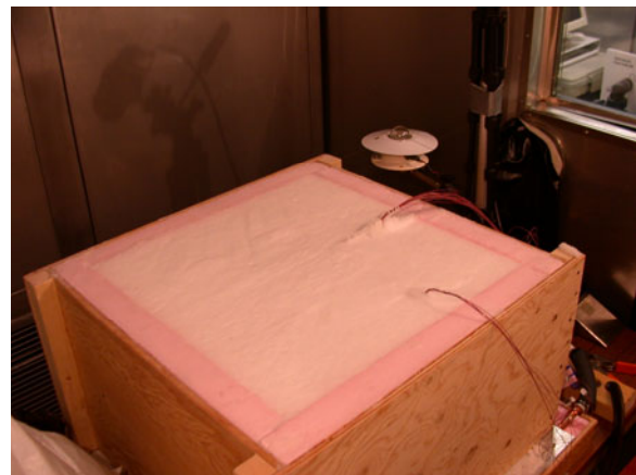
Figure 3: Insulated snow box with Eppley PSP and thermocouple arrays shown. Aluminum plate below box is the bottom boundary condition.
