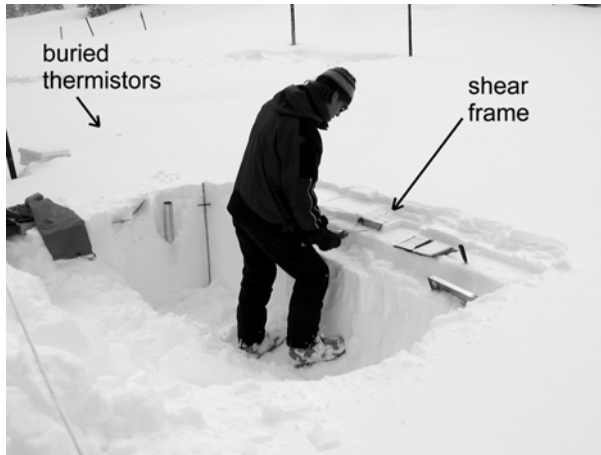
Fig. 7. Photograph of operator performing a shear frame test on a layer of facets on a crust. The bottom of frame is placed a few millimetres above the facet-crust interface and pulled to fracture within a second. The layer being tested was buried 2004-01-14 at Mt. St. Anne.
