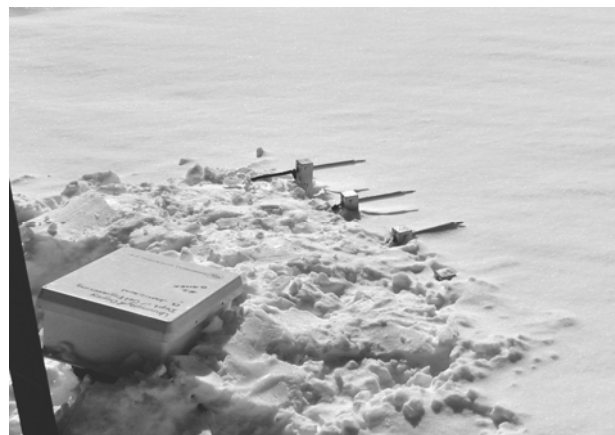
Fig. 6. Photograph showing three vertically oriented pairs of thermistors that were placed in wet snow before dry snow fell. Only the top thermistor of each pair is visible above the dry snow. The thermistors are connected to a datalogger in the white box that reads each temperature every two minutes and records the average temperature of each thermistor every hour.
