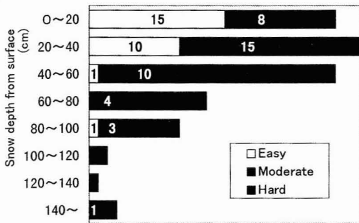
Fig. 9: Depth of failure plane
