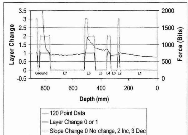
Figure 6 Pattern recognition of the layers
