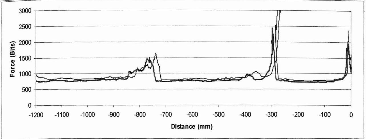
Figure 10 Correlated Force Distance profiles for two pushes
