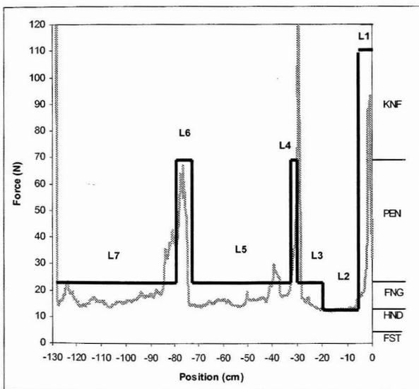
Figure 11 Snowpit test confirmed the ability of the probe to detect thin hard layers
