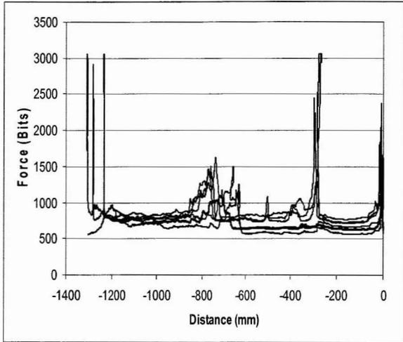
Figure 12 Multiple two dimensional probes taken at equal distances across the slope
