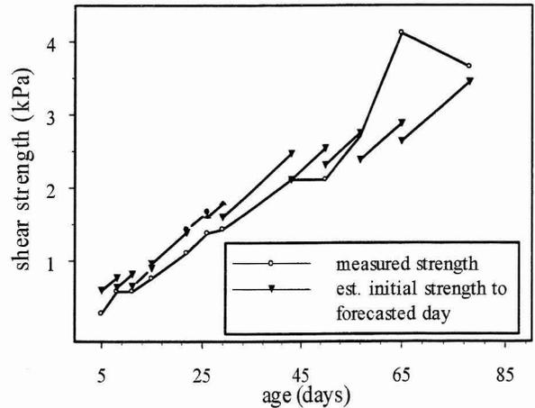
Figure 3: Model testing to forecast shear strength at Mt. St. Anne (faceted layer formed 07 January 2002)
