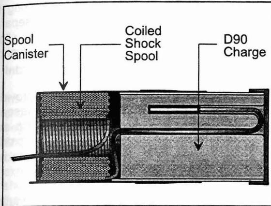
Figure 7: Section through a D90 booster (hand charge) fitted with a spool canister carrying 23m of shock tube.
