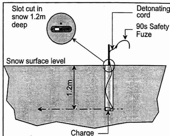
Figure 2: Charge set-up for experimental firings in stable snow pack.
