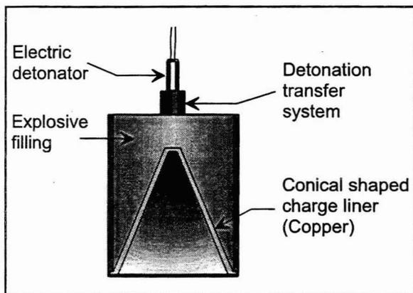
Figure 1a: Principal components of a conical shaped charge
