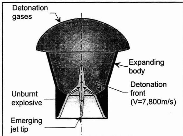
Figure 1b: Early stage of the liner collapse process 5 microseconds after initiation.
