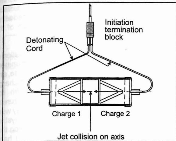
Figure 5: Paired charge configuration comprising 2 scaled down charges (Type 1 shown) co-axially arranged such that the jets collide upon simultaneous charge detonation.
