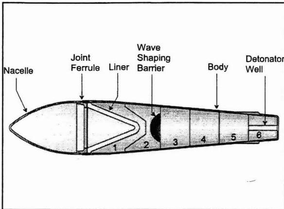
Figure 9: Section through the Mk I Avalanche Control Charge.
