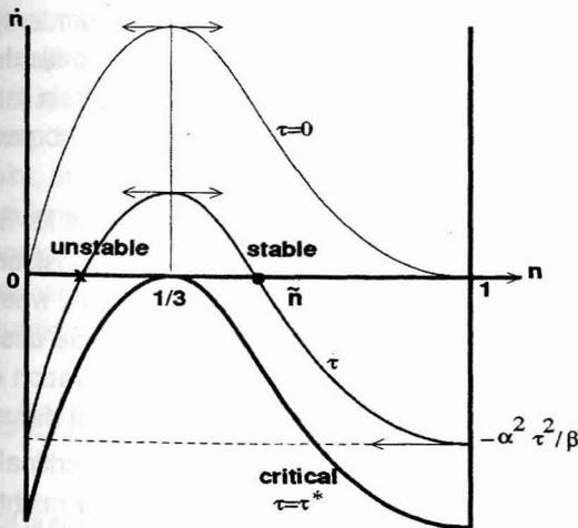
Figure 2: Schematic variations of the balance between welding and rupture rates as a function of the proportion of unbroken bonds  $n$ , at zero stress (upper curve), in the general case (intermediate curve), and in critical avalanche release conditions (lower curve).
