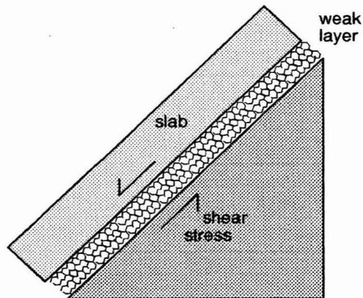
Figure 1: The weak layer is treated as an open cell foam made of a network of ice bonds. Under shear loading, it experiences creep flow through a balance between bond rupture and rewelding events.
