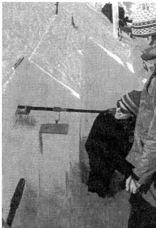
Figure 4. Bench mode test following shear fracture. The 0.04 \text{ m}^2 load plate is shown.
