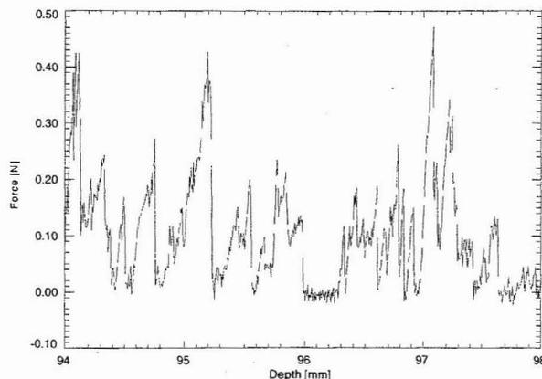
Figure 3: Force signal measured in faceted temperature gradient metamorphosed.
