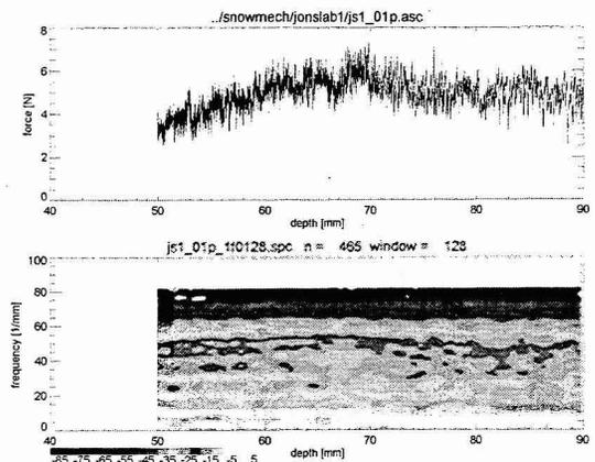
Fig. 9: Force signal and spectrum of a measurement where a failure occurred at depth 65 mm. The spectral bands seen above 65 mm disappear at this depth.
