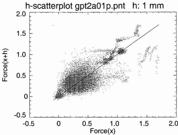
Fig. 4: H-scatterplot with a lag distance ( $h$ ) of 1 mm. It shows the spatial relationship of the force values at the location  $x$  to the force value at the location separated by the distance  $h$ .
