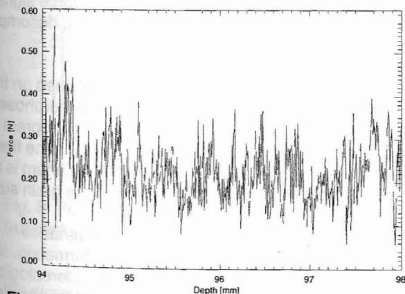
Figure 2: Force signal measured in round-grained decomposed snow.
