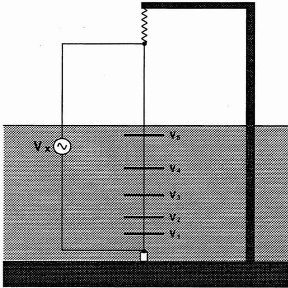
**Figure 1.** Apparatus for measuring settlement within snowpacks.
