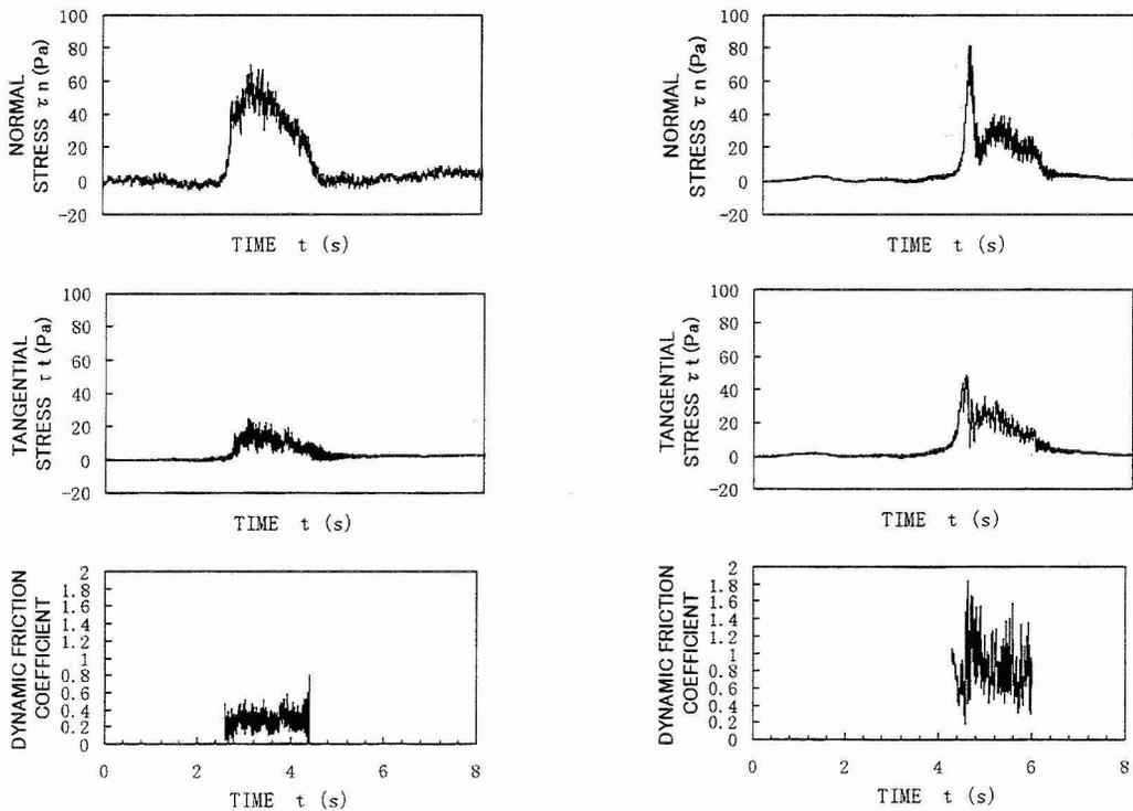
Figure 8. Normal stress, tangential stress and dynamic friction coefficient of a table tennis ball avalanche. The left column shows data obtained by the upper drag meter. The right is from the lower one.
