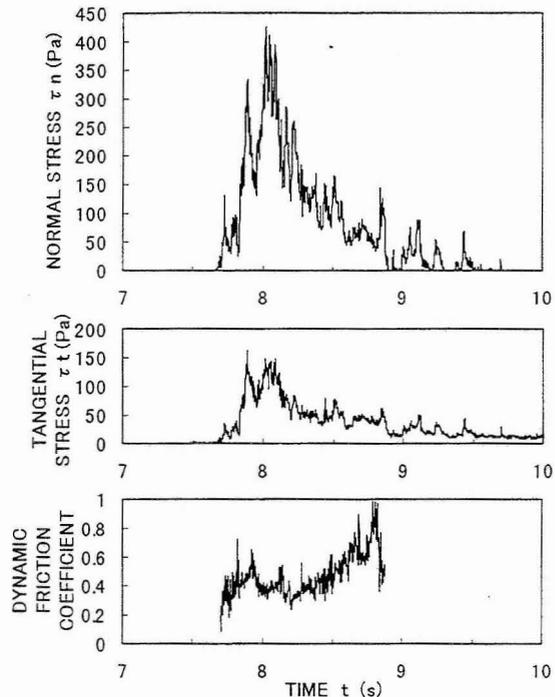
Figure 5. Normal stress, tangential stress and dynamic friction coefficient of a snow avalanche. Mass of snow released was 92 kg.
