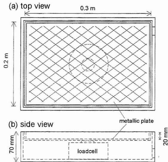
Figure 2. Top view (a) and side view (b) of the drag meter.
