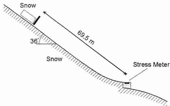
Figure 1. Schematic diagram of the experimental set-up for snow avalanches. Side view.
