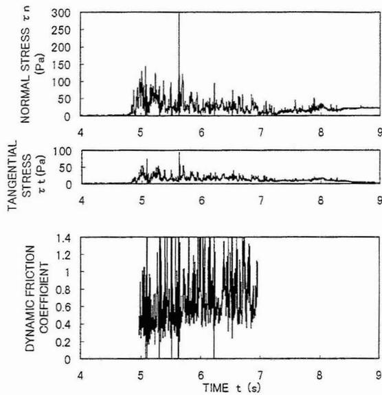
Figure 4. Normal stress, tangential stress and dynamic friction coefficient of a snow avalanche. Mass of snow released was 46 kg.
