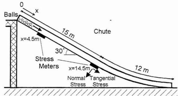
Figure 3. Schematic diagram of the artificial chute. Side view.
