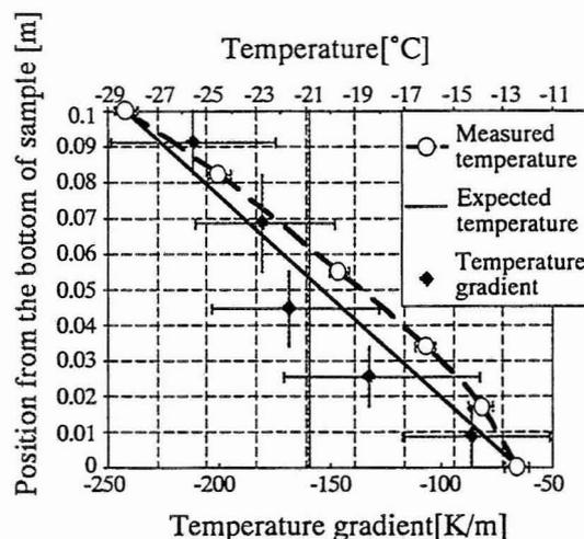
Figure 3. Temperature distribution and temperature gradients in snow sample
