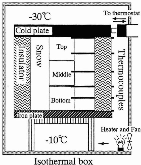
Figure 2. A schema of apparatus
