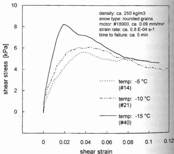
Fig. 4 Example of stress-strain curves for three different test temperatures:  $-5$ ,  $-10$ , and  $-15^\circ\text{C}$ . Snow stiffness in these examples is about 200, 300 and 600 MPa, for  $-5$ ,  $-10$ , and  $-15^\circ\text{C}$ , respectively.
