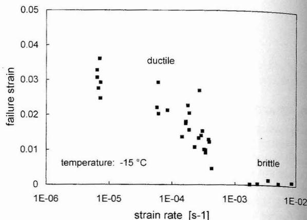
Fig. 3 Failure strain vs. strain rate; test temperature:  $-15^\circ\text{C}$ .
