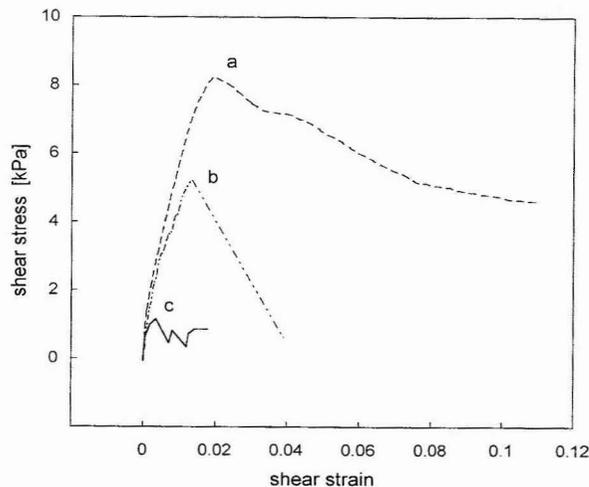
Fig. 2 Example of stress-strain curves for three different strain rates, (a):  $6.1 \times 10^{-5} \text{ s}^{-1}$ , (b):  $2.7 \times 10^{-4} \text{ s}^{-1}$ , (c):  $2.3 \times 10^{-3} \text{ s}^{-1}$ ; test temperature:  $-15^\circ\text{C}$ .
