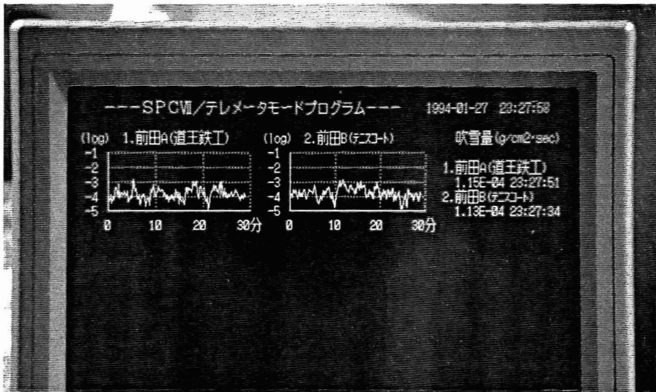
Photo 4 Real time display of blowing snow data at two Maeda sites telemetered to the Ishikari observation site
