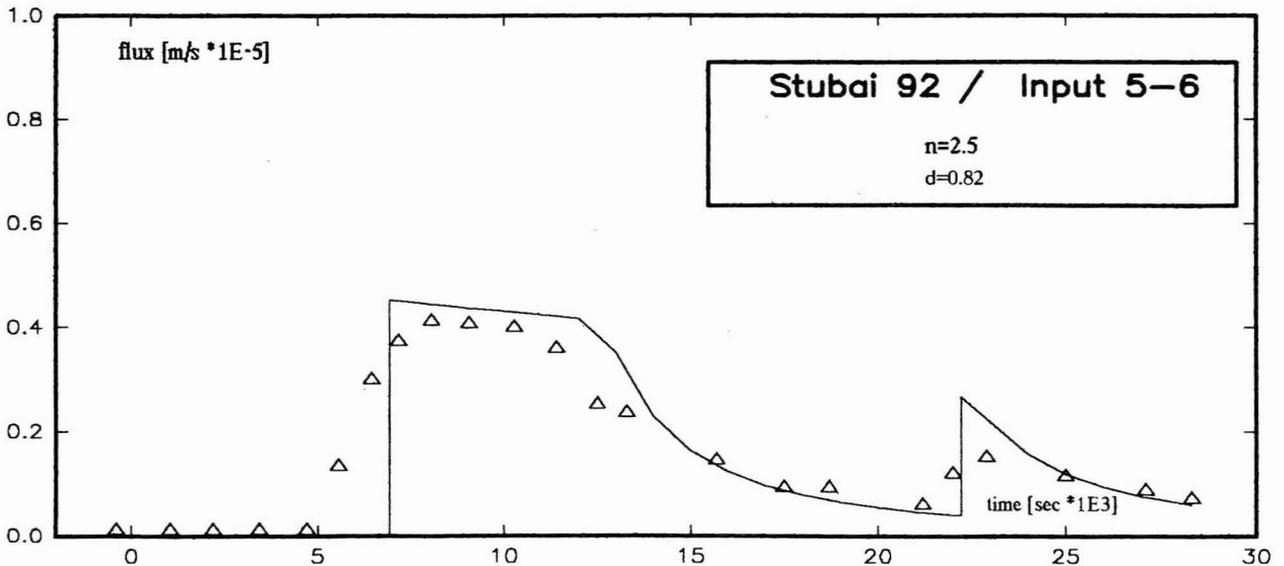
Figure 3 - Measured data points of the output flux and according modelling at a depth of 1.38m
