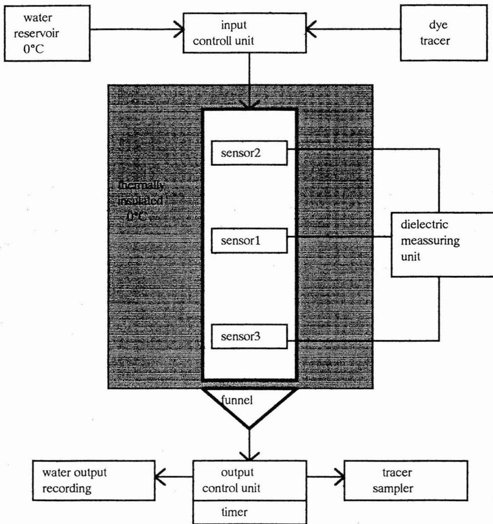
Figure 1 - blockdiagram of the experimental setup
