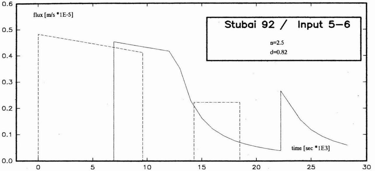
Figure 2 - Two water inputs and the according modelling of the output flux at a depth of 1.38 m
