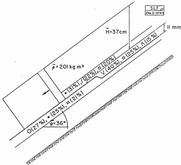
Figure 5: Mean slab configuration and most often observed grain forms, either as weak layer or as weak interface and as upper and lower adjacent layer.
