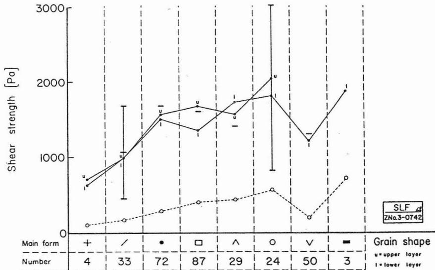
Figure 6: Mean and minimal values of shear strength for main grain shapes. The mean values in weak layers are given by horizontal bars (besides two values of stand. dev.). The measured mean values at interfaces are denoted by dots. The minimal values are denoted by small circles.
