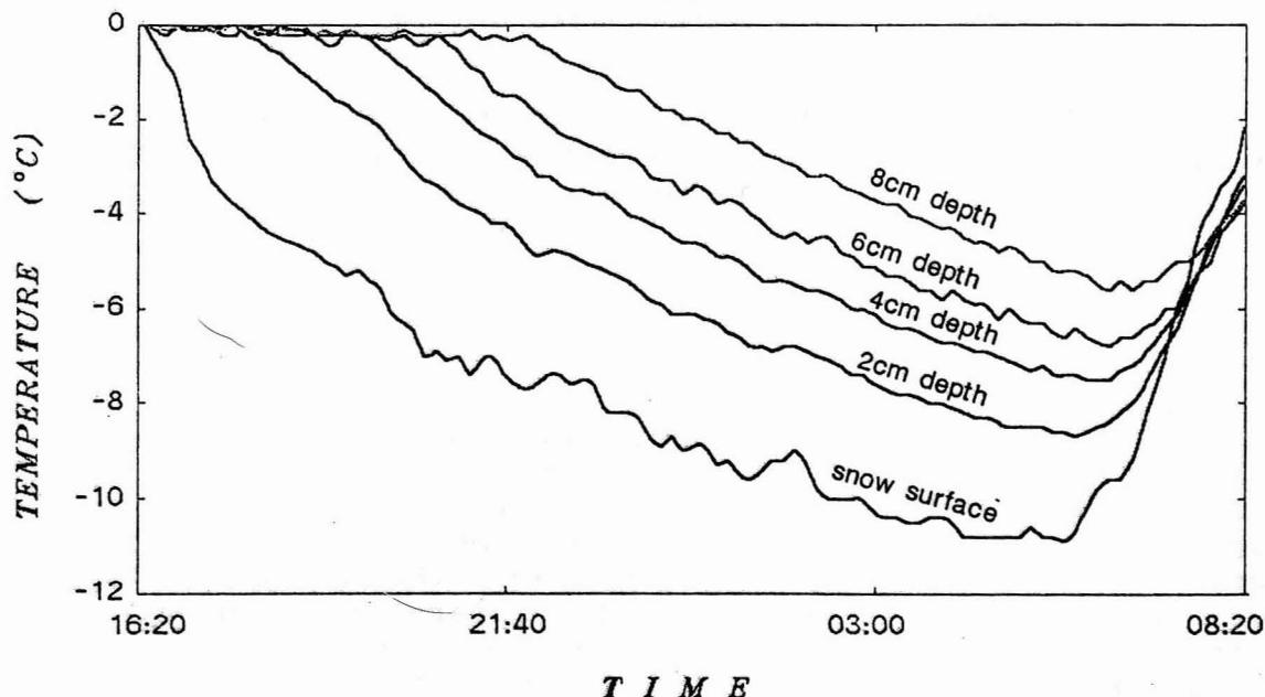
Fig. 3. Snow temperature profile at every 2cm from surface to 8cm depth during the night time of 2-3 March, 1990.
