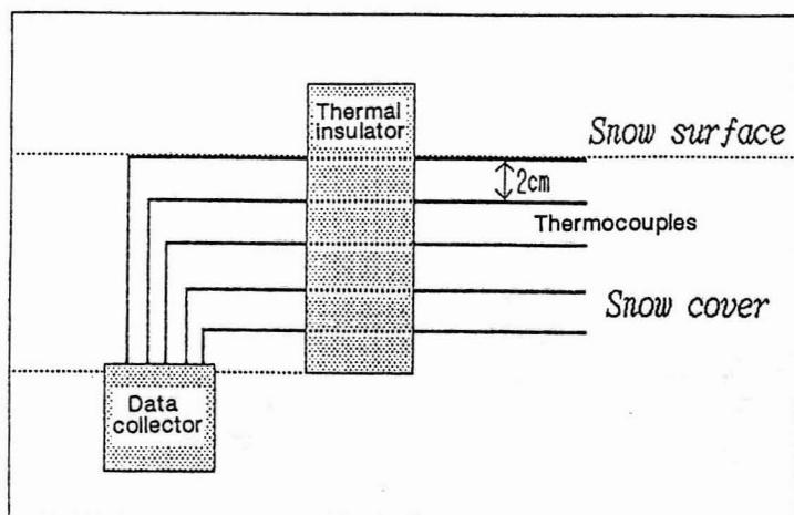
Fig. 1. A device for measurement of snow temperature.
