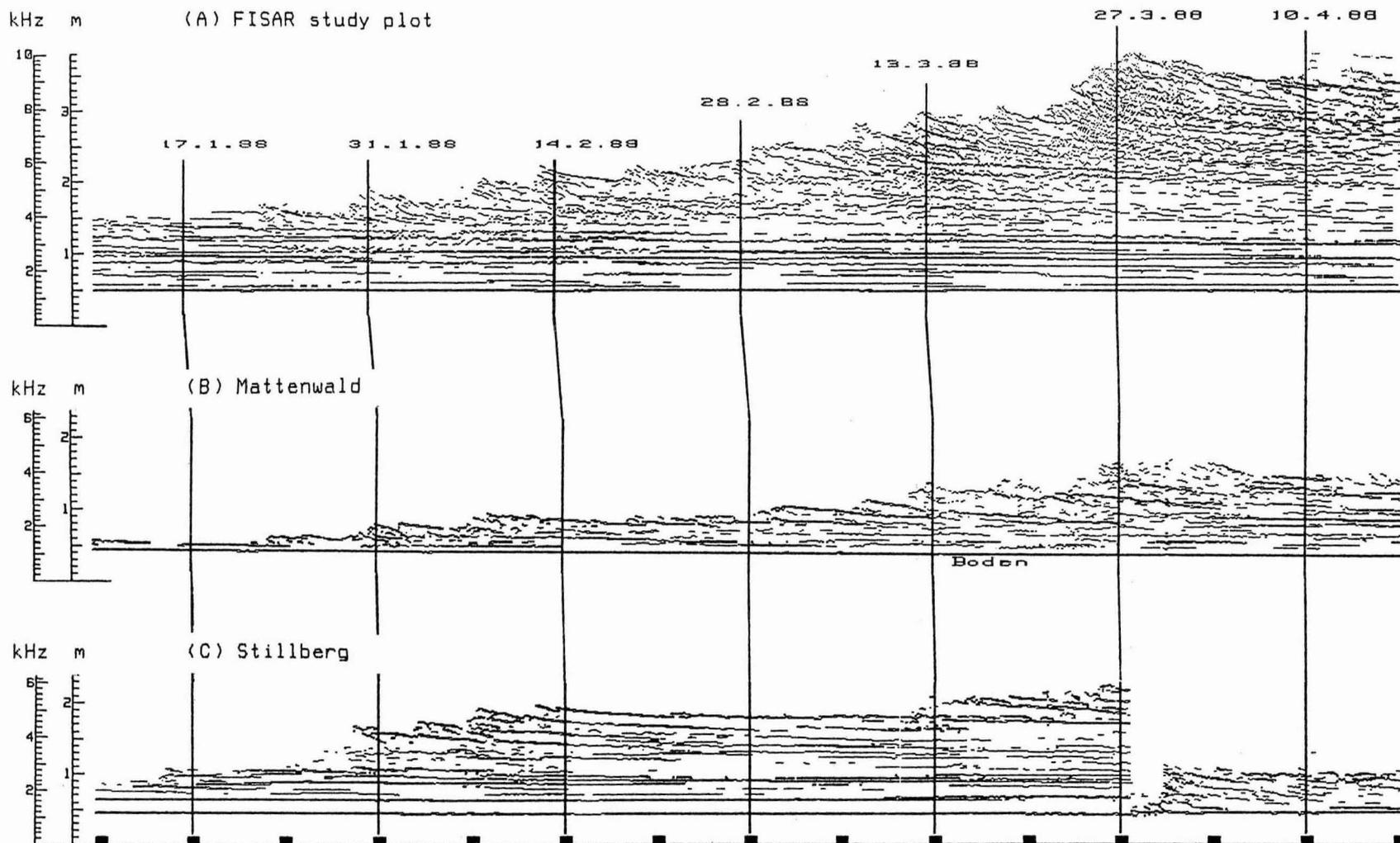
Figure 1 Bitmap representations of electromagnetic snow cover profiles (mid January to mid April 1988) from X-band FMCW radars at FISAR study plot (A) and starting zones Mattenwald (B) and Stillberg (C). Markers are plotted every Sunday, date is given in European format. An approximate height scale is given in addition to the frequency scale.
