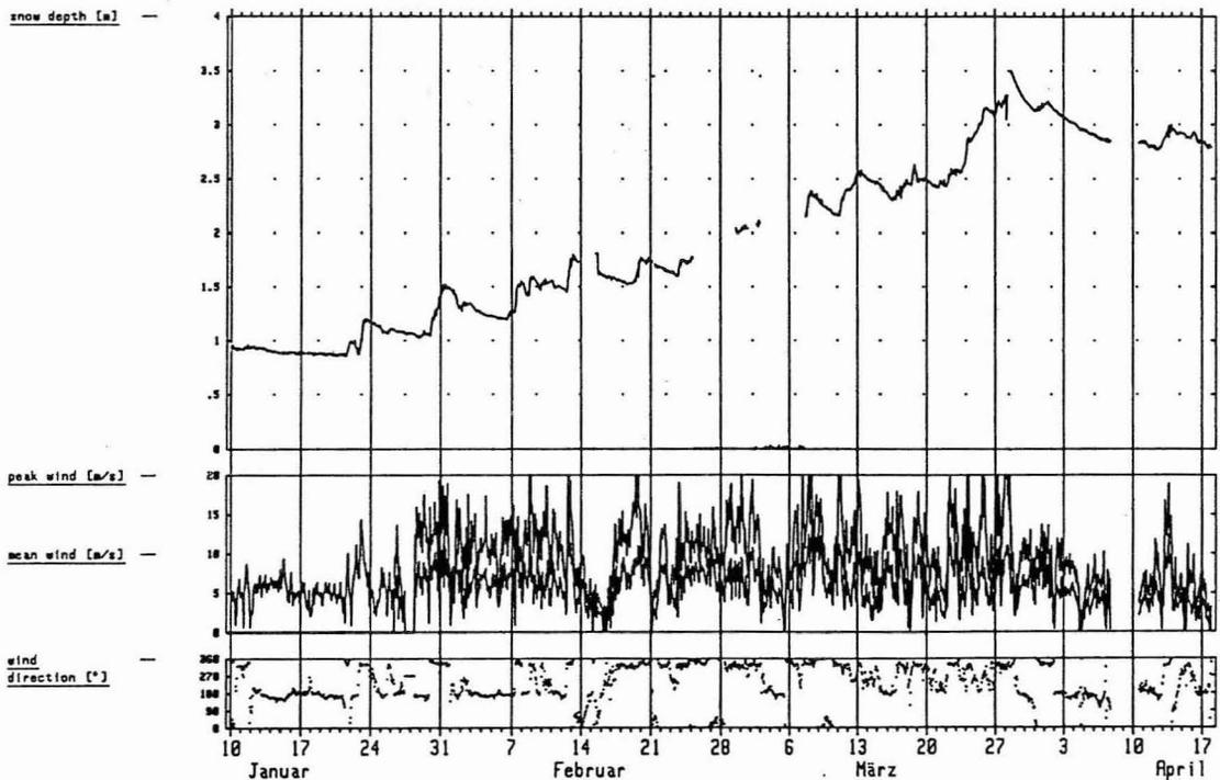
Figure 4b Wind and snow depth data (ultrasonic gauge) from Weissfluhjoch.
