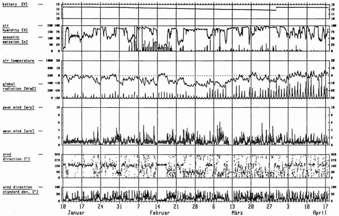
Figure 4a Meteorological data from Mattenwald logger.
