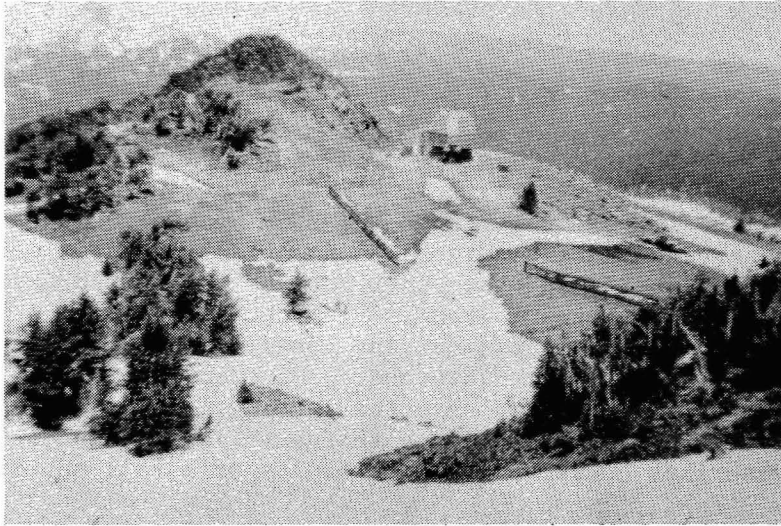
Figure 2 A 1.2-m snowfence near the top terminal of Pine Marten lift did not accumulate enough snow to cover the wind-swept area during the 1986-87 season.
