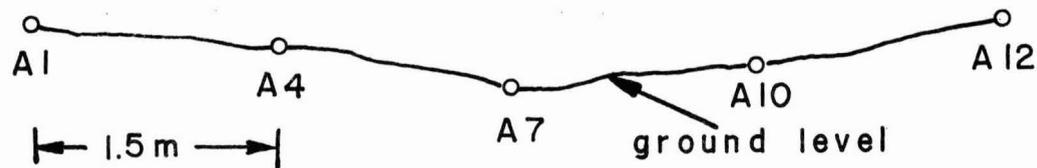
Figure 1. The array of thermistor strings installed to monitor snowpack temperatures. The grid defines the spacing of the thermistors in relation to each other and the original snow surface. These were installed on a southwest exposure similar in aspect, angle, and elevation to a slope which constituted the major hazard to the pipeline work site.
