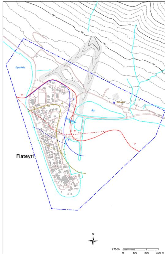
Figure 2. The hazard map for Flateyri before and after the construction of two deflecting dams.
