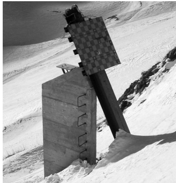
Figure 2: Instrumented structure set up in path n°2. The 1 m² plate can be moved along the beam to be located exactly at the surface of the snow-cover.
