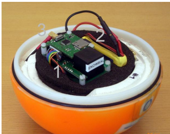
Figure 2: (1) IMU, Internal Measurement Unit equipped with several sensors. (2) Power supply. (3) GPS antenna.
