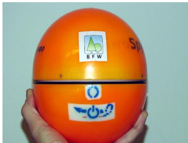
Figure 1: Exterior view of the Snowball. The sensors can be activated with a magnetic switch (bottom half of the sphere) from the outside without opening the ball in the held.
