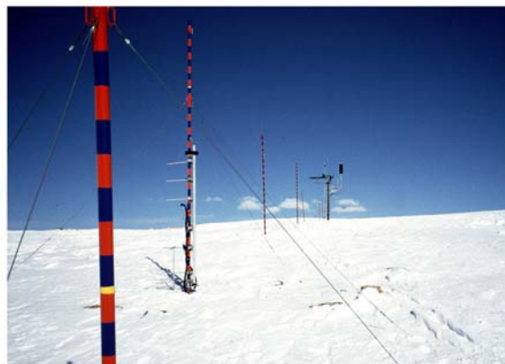
Figure 4: Partial view of the horizontal profile of snow depth on both sides of the pass.
