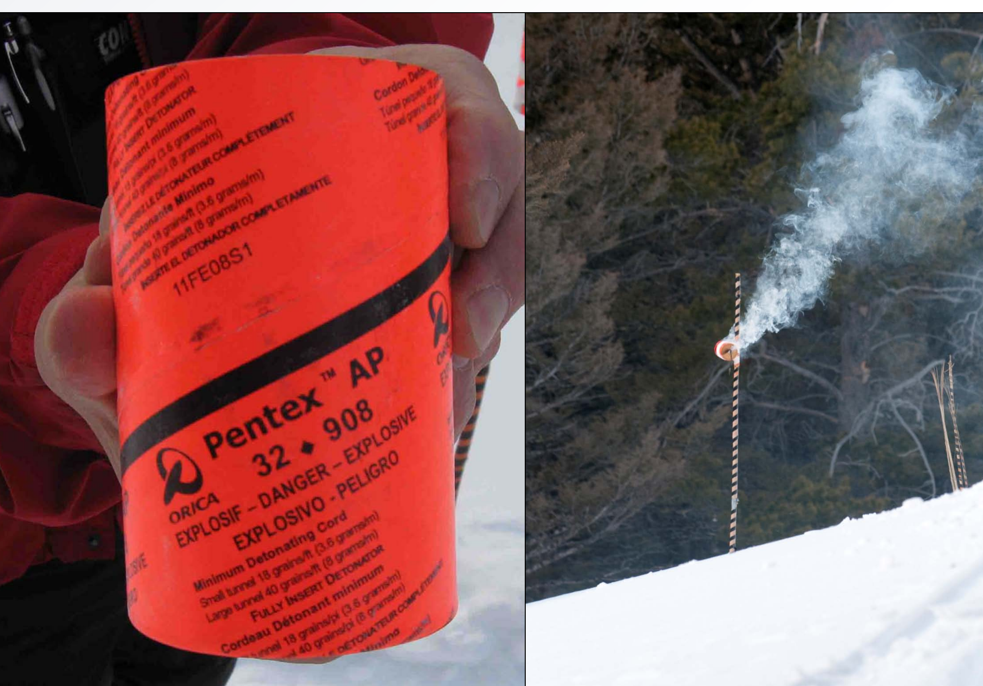
Figure 2. Left: 0.9kg Pentolite cast booster. This charge was used for several test configurations. Right: 0.9kg booster suspended 1m above the surface of the snowpack.
