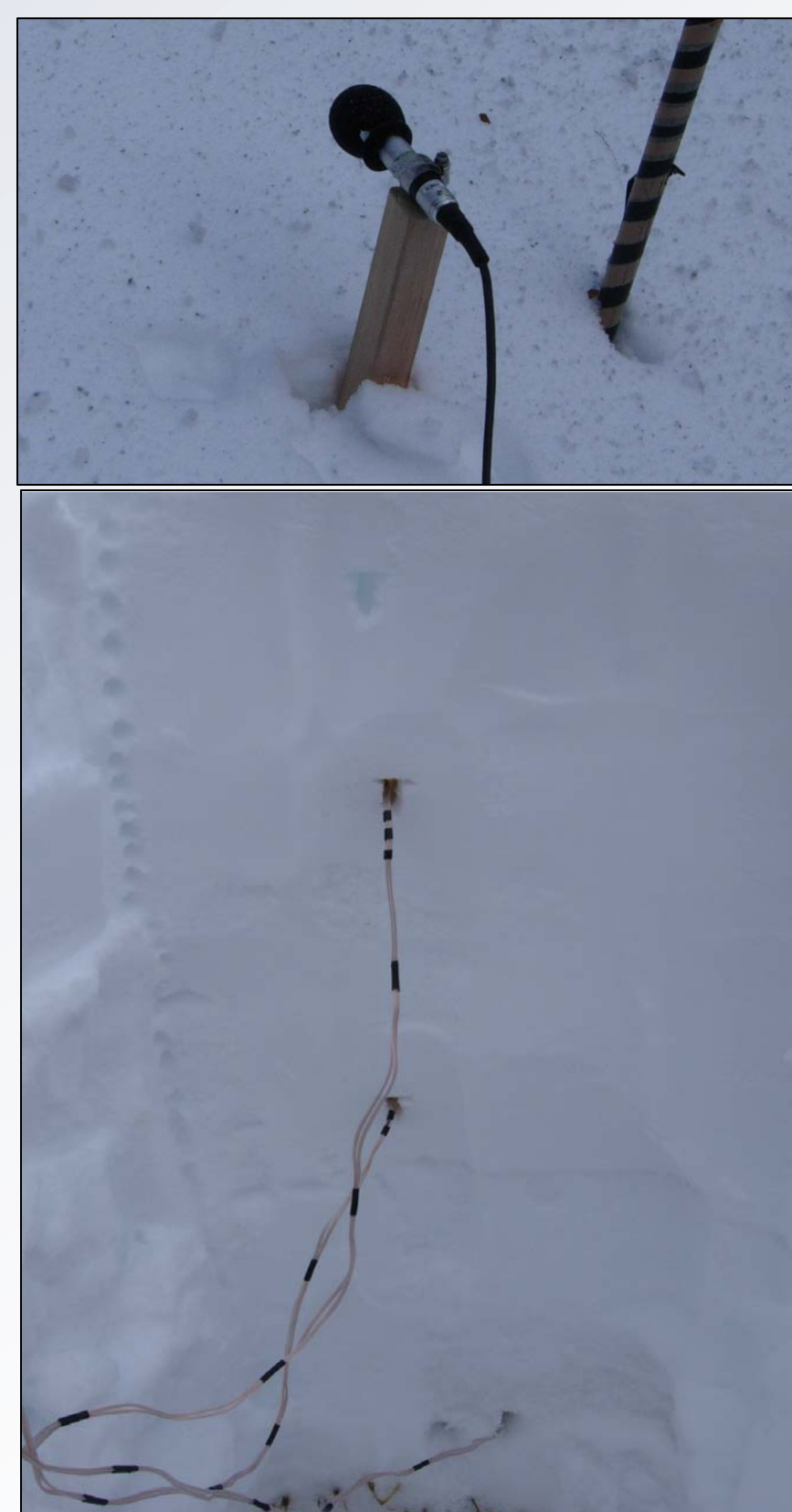
Figure 5. Top: Larcor ± 34.4 kPa air overpressure sensor. Lower: Accelerometers placed through the depth of the snowpack. Pits were later backfilled with loose snow following placement.
