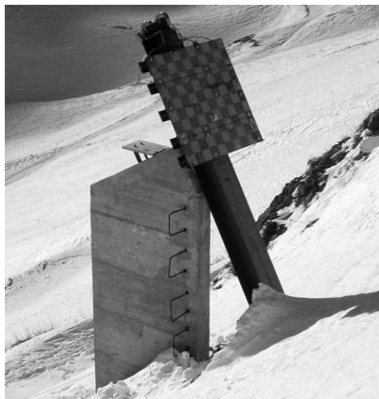
Figure 3: Instrumented structure set up in path n°1. The 1 m 2 plate can be moved along the beam to be located exactly at the surface of the snow-cover.
