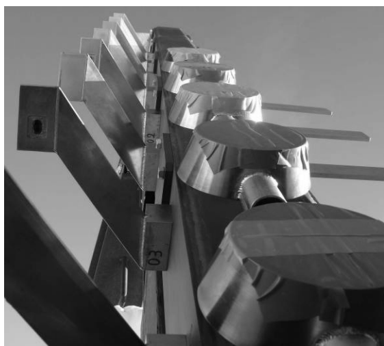
Figure 5: Pressure (right) and velocity (left) sensors set up on the tripod at path n°2.
