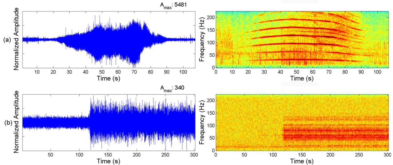
Figure 3: Two examples of background noise. (a) Helicopter. (b) Wind. Left panels: waveform. Right panels: running spectrum of the data. The colors indicate intensity, from dark blue (low) to red (high).
