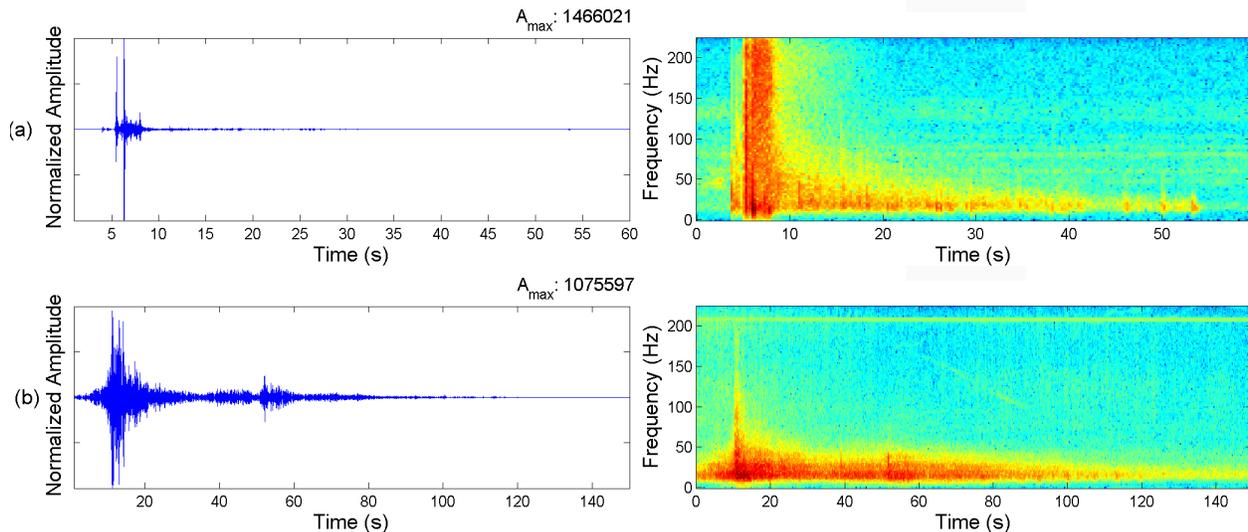
Figure 4: Two examples of signals generated by avalanches. (a) Slab avalanche. (b) Loose snow avalanche. Left panels: waveform. Right panels: running spectrum of the data. The colors indicate intensity, from dark blue (low) to red (high)
