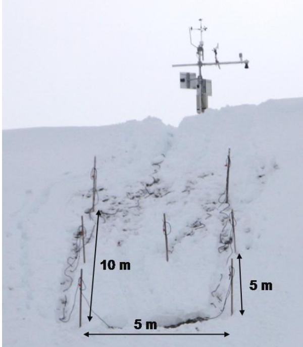
Figure 2: Photo of the deployment configuration for the winter of 2009-2010. The cables of the data acquisition system were fixed to the ground early in the season. Wooden posts were fixed in the ground in order to be able to connect the sensors once the cables were buried by snow.
