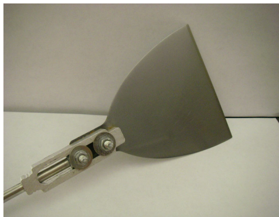
Figure 1. Paint scraper blade, showing attachment to threaded rod using an aluminum turnbuckle and two bolts.
