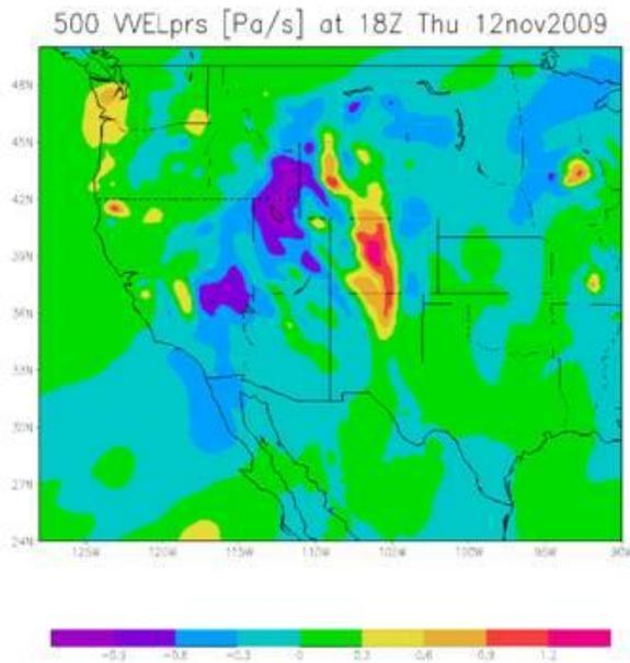
Figure 9: 500mb vertical velocities. Negative numbers indicate upward vertical motion (UVM); note core of UVM in northern Utah southeastern Idaho, western Wyoming, and southern Montana. Phasing of UVM and humidity can generate copious convective precipitation.
