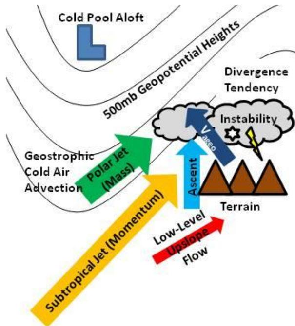
Figure 14: Conceptual diagram of convective snowfall events arising from unbalanced ascent and ageostrophic flow ( $V_{ageo}$ , dark blue arrow) via phasing of the STJ, PJ, and upper level low pressure trough. Clouds indicate the region of maximum likelihood for convective precipitation.
