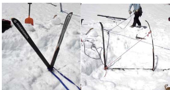
Figure 11: The photo on the left shows skis in as a X. This failed at 2.2 kN in pencil hardness snow. The photo on the right is two skis in line at the point of failure at 2.8 kN. A noticeable bow has formed in the front ski.
