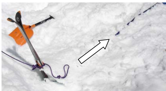
Figure 12: a pair of skis as a mid clip is shown just prior to failure in shear. Note the tension crack. The skis were in to 850 mm and failure occurred at 14.8 kN in pencil hardness snow that had been compacted in front of the skis.
