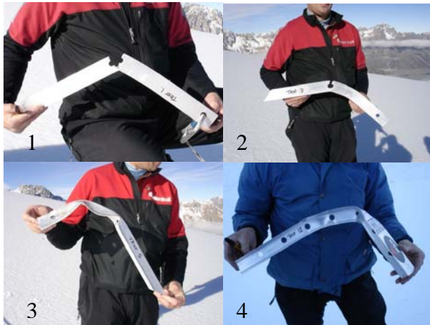
Figure 5: Four upright top clips in knife hardness - 10^{\circ} C snow. 1: Al alloy (6261 T6) failed in shear at 9.4 kN. 2: Softer Al alloy failed in compression at 6.7 kN, 3: Was open part of V to load and failed at 4.4 kN through bending of the stake. 4: MSR coyote that failed in compression at 7.8 kN. Bogie (2005)
