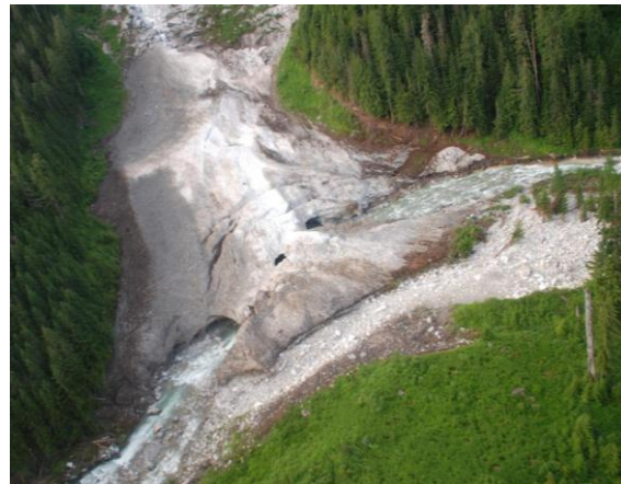
Fig. 5. Montrose Intake and Path MS-6, May 2008 avalanche event (Jun. 26, 2008 Photo). Deposit blocked Montrose Creek with a thickness up to 20 m which persisted well through the summer.
