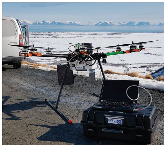
Figure 1: UAV-borne radar system. The UWiBaSS is the grey box mounted beneath the drone, with the transmitting antenna (grey plate) and both receiving antennas (black sheets) visible.
