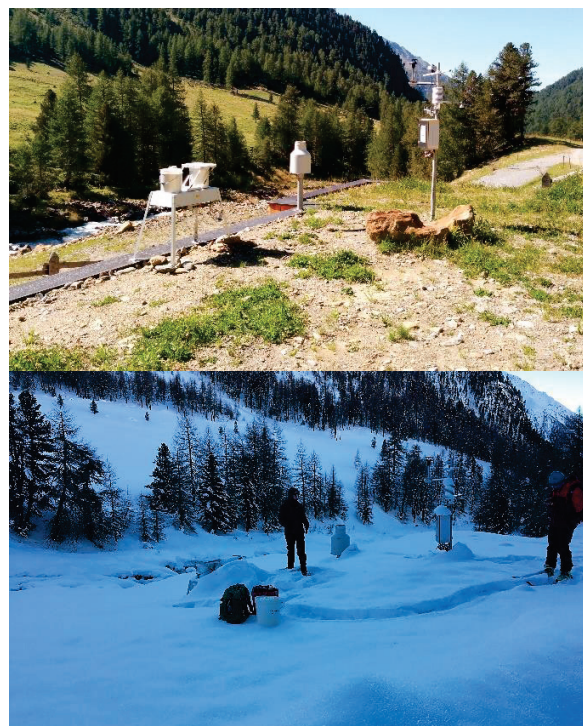
Figure 1: Picture of station M4s, composed by a meteorological station, a snow height sensor, a weighting pluviometer and an atmospheric deposition sampler. Above the station on August 24 th 2017, below on January 15 th 2018, after being hit by a powder avalanche.
