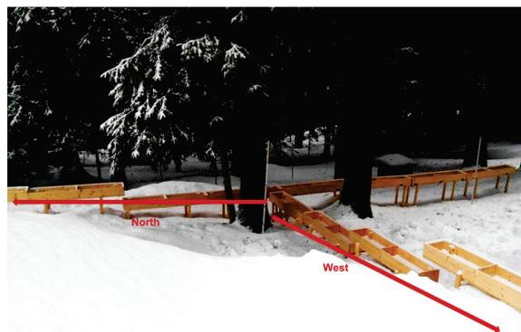
Figure 2: Snow interception measurement device.
