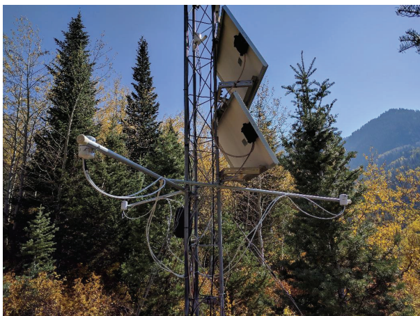
Figure 5: Goniometer Mounted on Mid Canyon Tower
