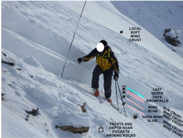
Fig. 07: The snowpack at the avalanche crown in the skied area. Compare with Fig. 05 and 06. The snowpack is considerably thinner and note the facets and depth hoar pockets around the protruding rocks.
