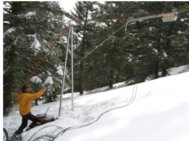
Fig. 4. GPR profiles from an aerial tramway were performed weekly to monitor major stratigraphy, SWE, and depth.
