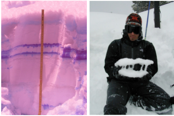
Fig. 2. Dye experiments indicate water can move hundreds of meters downslope along layer boundaries on time scales of hours, often with vertical melt pathways occurring between multiple saturated layer boundaries. Snow between vertical melt channels is typically close to dry, while channels have high liquid water content. Right photo: Adam Brown.
