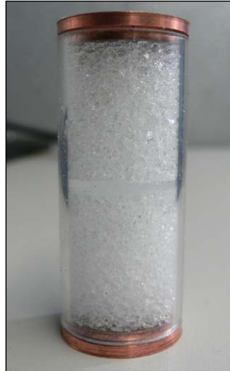
Fig. 2: Ice/snow sample with a 2 mm thick ice lens placed between natural snow of mean diameter 2.5-3 mm.
